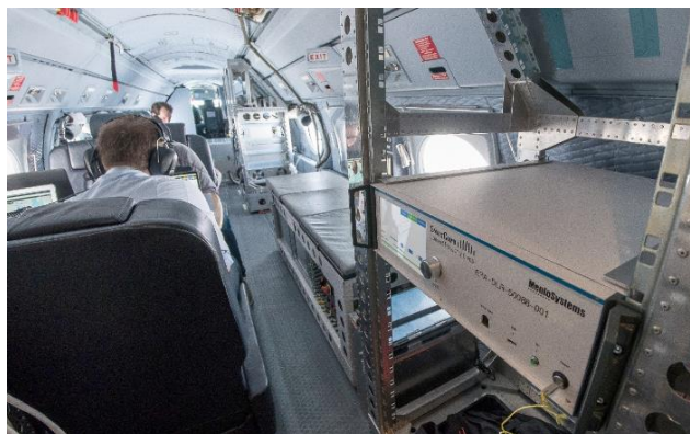
The world's first airborne frequency comb on a mission to enable a LIDAR-based greenhouse gas monitoring campaign – employing figure 9® technology.
